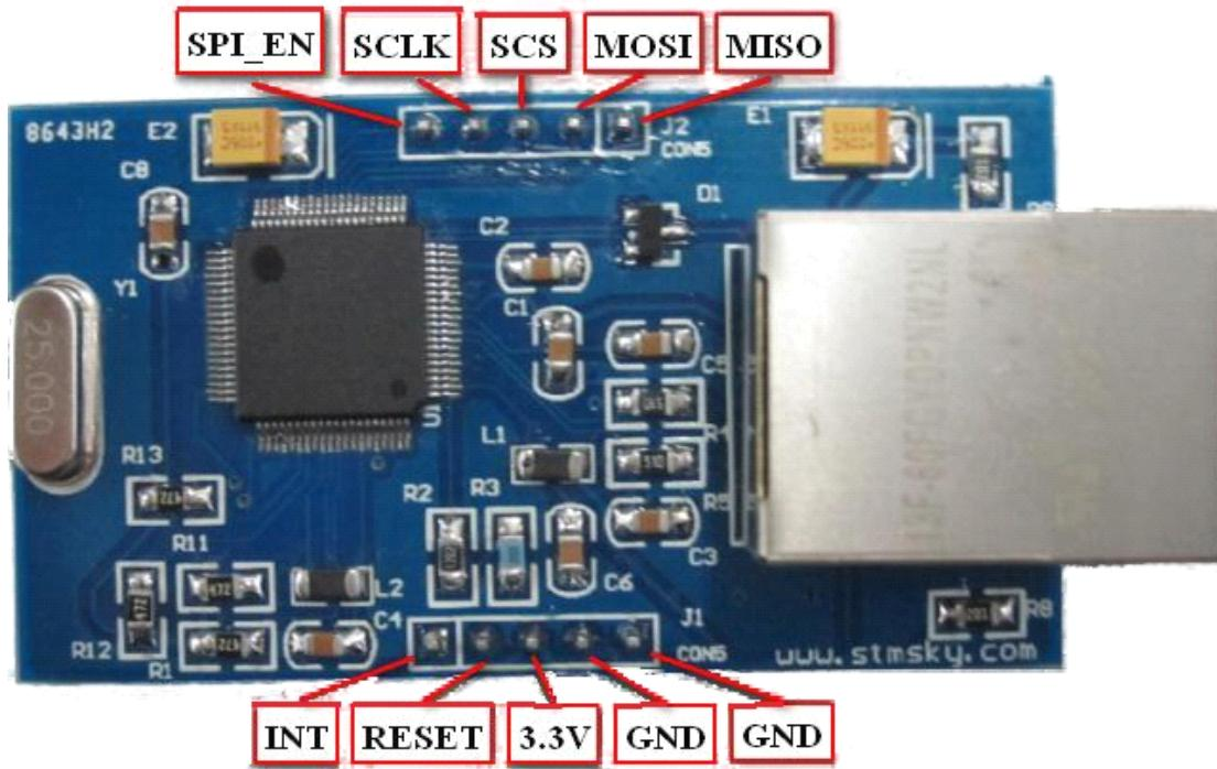
To use it on the Arduino, you just connect the SPI\_EN pin to 5V or 3.3V with a pull-up resistor, connect SCLK, SCS, MISO, MOSI to the SPI port of Arduino, connect the INT pin to the digital 2 of Arduino, connect the RESET pin to the RESET of Arduino, and
