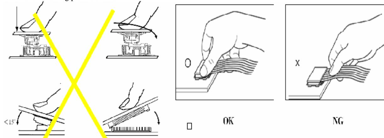
**Precaution for soldering the LCM**
