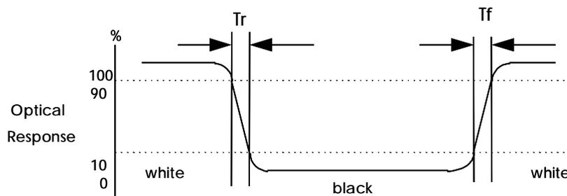
The values specified are at an approximate distance 500 mm from the LCD surface at a viewing angle of  $\Phi$  and  $\theta$  equal to  $0^\circ$ . Measurement condition : Refer to next pages ( B - light source , Halogen Lamp, with polarizer )
